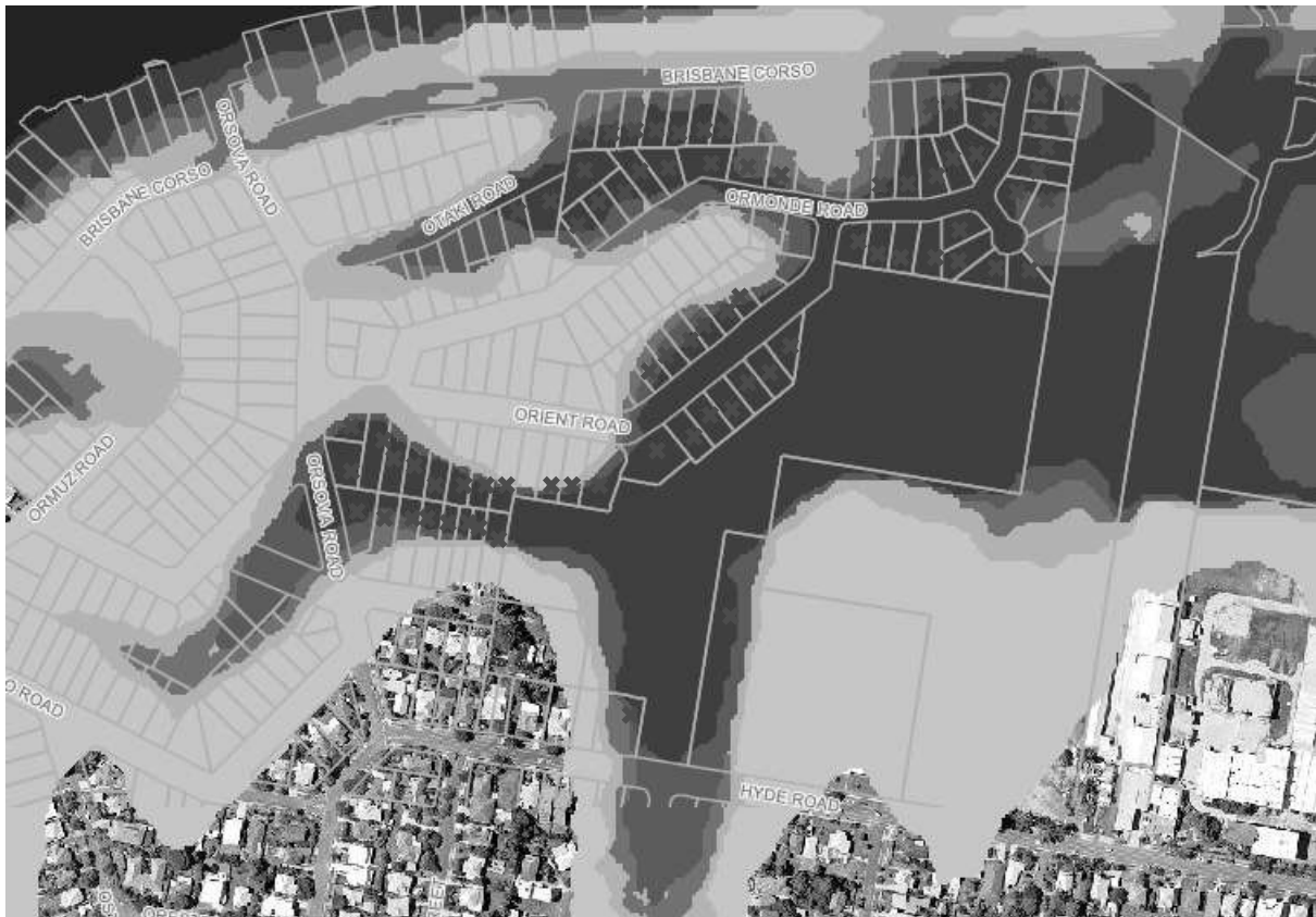
Figure 5 - Affected properties due to illegal filling & drainage (BCC flood mapping)
